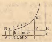
vided into portions, which shall be as the increments of the velocity in equal times, therefore A k, A l, A m, A n, &c. will  $\alpha$  velocity, and therefore  $\alpha$  resistances at the beginning of the respective times.
